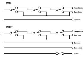
Note: Circuits shown with magnet in secure position.
